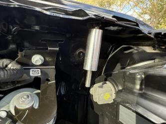
2. The catch can will mount off the fender bolt on the driver side close to the headlight. Screw the provided aluminum stud assembly onto the bottom of the fender bolt, and tighten it using the allen wrench.
