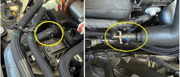
1. Locate the factory PCV hose and remove it. The hose will connect from the top of the valve cover to the front side of the intake manifold. The fittings at each end of the hose will have quick connect fittings that are released by moving the lever to the side, then sliding the fitting off of the engine.
