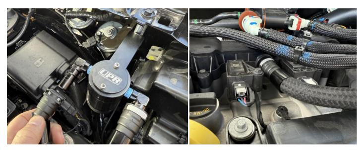
5. Install the PCV hose from the opposite side of the catch can to the PCV fitting on the valve cover. The 45 degree fitting will connect to the catch can, and the straight fitting will connect to the PCV fitting.
