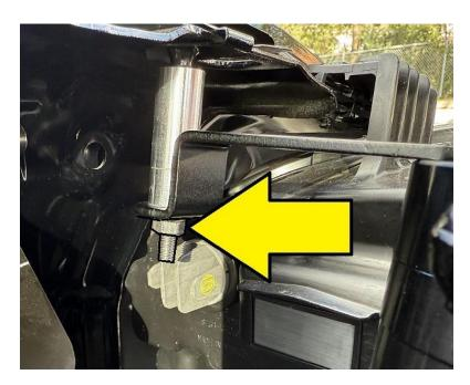
3. Install the catch can bracket onto the stud with the provided 10mm nut. The catch can should be mounted so that it faces the engine. Tighten the nut with a 10mm wrench.
