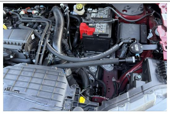
6. Route the hoses so that they avoid any under hood hazards. Check your connections and verify that the catch can bracket is secure.
