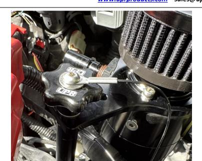
3. Install the UPR 5050 catch can onto the mount and secure it with the supplied knob.
