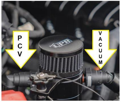
4. The PCV side of the catch can will be facing towards the back of the engine compartment. The Vacuum side will face forward and will have a silver marking on the male fitting.
