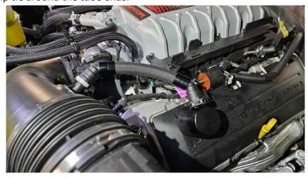
8. Install the CSS with the supplied hose assembly. When installing the CSS, be sure the collar on the bottom is pulled up, it will snap when seated onto the fitting.
