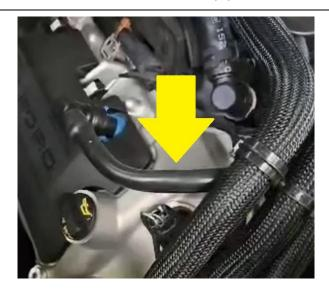
5. Locate the factory PCV hose that runs from the passenger valve cover PCV valve to the Supercharger vacuum port. Remove the factory fittings by pushing the blue tabs on the fittings to the side and lift the hose off.
