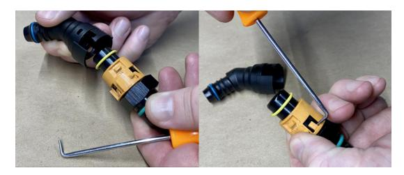
\* If you want to return your vehicle back to stock, you can replace the fittings on the driver side hose with UPR part number 2025-39 and 2025-40. Use a heat gun or lighter to gently warm the plastic tube – do not melt or burn the tube. Pull the fitting out of the tube once it is warm, and insert the new fitting into the tube while it is still warm. The tube will conform to the fitting as it cools. To assist, you can wrap a small zip tie around the tube ends.
