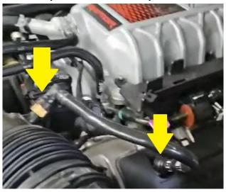
7. To install the Clean Side Separator (CSS), you will need to remove the orange fittings on the driver side Crankcase vent hose. These fittings are not a quick release style. The process below will illustrate how to remove the fittings. The fitting is shown off of the vehicle so we could show the best view.
