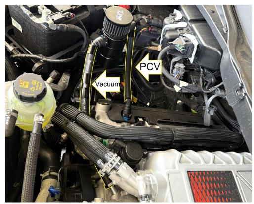
6. Connect the longer hose from the vacuum side of the catch can to the intake manifold vacuum fitting on the supercharger vacuum fitting. If you selected to add a Pro Series Check valve, be sure the arrow printed on the check valve faces away from the catch can. Connect the PCV side to the PCV valve on the passenger side valve cover.
