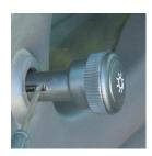
Remove the factory headlight knob by sliding a small flat head screwdriver into the slot on the side of the headlight knob. Pry the factory clip towards you, then pull on the headlight knob. It should slide off the stem.
