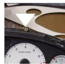
Once the speedo cluster is removed from the car, place it on a desk or flat surface to begin the White Faced / EL installation. Remove all of the gold colored retaining screws that surround the outside of the clear / black plastic housing. The black bezel and clear plastic should now be able to separate from the cluster.
