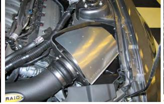
using the 1/4-20 Button Head Screws and Washers. toured edge going away from the filter. Start at the front NOTE: Installation of the Rain Shield is optional but of the vehicle and work your way back. Replace the enhighly recommended for vehicles with Power Dome gine cover. hoods with heat extractors.
