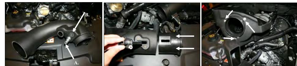
4. Install the Grommets and Fittings into the Airaid intake 5. Using the supplied Torx driver, remove the MAF sentube. A) All models will require the use of the 5/8" Fit- sor from the Factory airbox and create the Tube assemting and the 5/8"Grommet. B) Automatic transmission bly.
